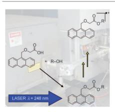
APLI application: Small molecules and polymers can be analyzed quantitatively by using atmospheric-pressure laser ionization (APLI) coupled to time-of-flight mass spectrometry. This is realized by a derivatization strategy that facilitates selective ionization of polar and non-polar compounds in complex matrices without hyphenated techniques or stable-isotopelabeled standards.
