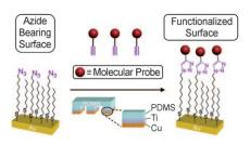
Minting a Stamp: The preparation of copper metal-coated elastomeric stamps and their use in catalyzing the Cu-catalyzed azide—alkyne cycloaddition reaction heterogeneously through microcontact printing is described (see scheme). This StampCat process is compared to other conventional surface-functionalization techniques, including traditional microcontact printing and solution—surface-based reactions.
