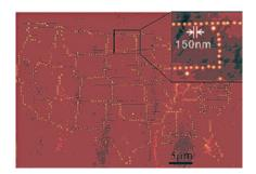
DPN benefits  $\mu$ CP: The intrinsic drawbacks in conventional microcontact printing, that is, roof collapse and lateral ink diffusion, were addressed by using topographically flat, chemically patterned PDMS stamps made by dip-pen nanolithography. The chemically patterned flat stamps were used for contact printing of various inks including thiols, proteins and hydrophilic dyes. The as-made features can reach sub-100 nm resolution and a very low filling factor (see AFM picture).
